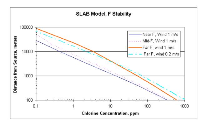
The "F Stability" is not the only stability that behaves this way. We can have an A Stability sliding into B, then C, and D or D sliding into E, than F as sunset and night time approaches.
